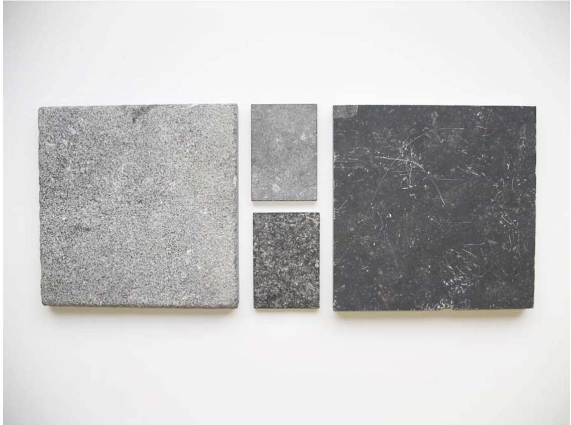
Figure 2. Four different finishes of the same Belgian Bluestone. Flamed finish at left is the roughest and lightest, while honed finish at right is the smoothest and darkest.
