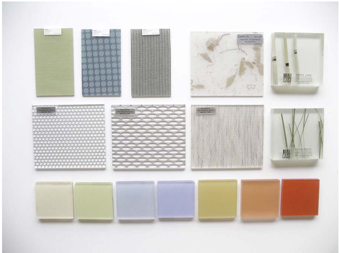
Figure 4. Fabric and natural forms laminated into resin materials are available in many colors.
