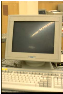
Illustration 12: Lights at service desks should be positioned so they do not reflect in computer monitors.
